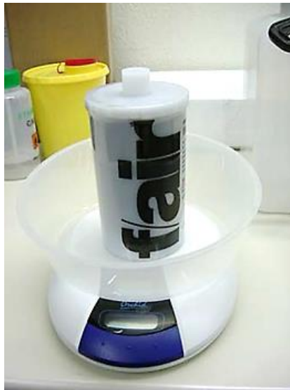
Figure 6: “Activated Charcoal Canister” Weighted to Assess if it needs to be changed
