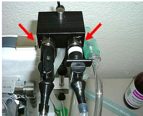
Figure 9: "Dual Diverter Manifold with the Left Output Open"
