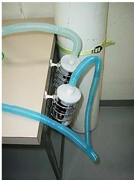
Figure 5: “Double Scavenging System with 2 Activated Charcoal Canisters”
